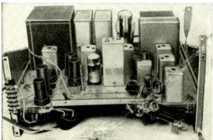
Converted BC-1068. R.f. circuits at right, sound channel at center.
