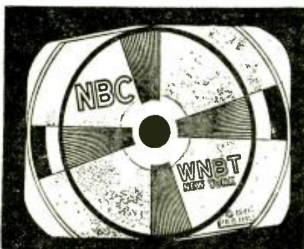
Fig. 7—Deflection yoke is improperly placed.
