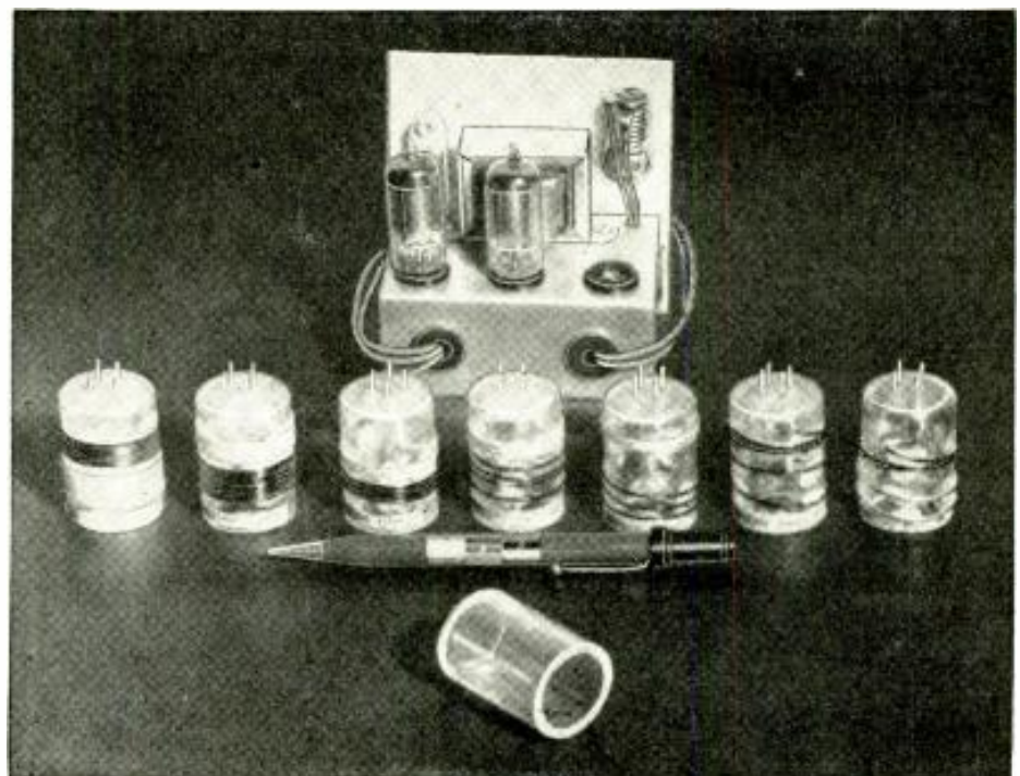
Rear-chassis view, with coils removed. The six shown cover the band from 5 to 100 meters.
